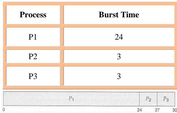
Figure-1 Process parameters and grant chart for FCFS. In the first Gantt chart, process P1 arrives first. The average waiting time for the three processes is (0 + 24 + 27) / 3 = 17.0 ms.
